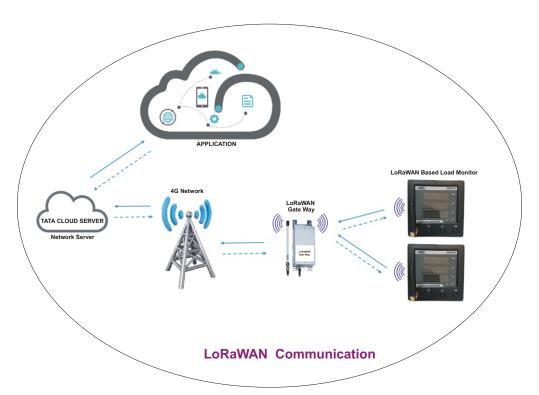
LoRaWAN network is typically set up in a star-of-stars topology, where gateways pick up the real time data payload broadcast by the our LoRaWAN based Load Monitor iLM8311PL and forward them over an Internet Protocol (IP) based network to a network server.
